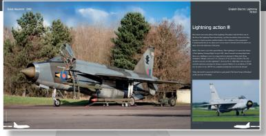
The Lightning was the only aircraft that could be equipped with overwing external fuel tanks. Now there's a concept! Another unique aspect of the jet was that its two engines were placed one on top of the other!
